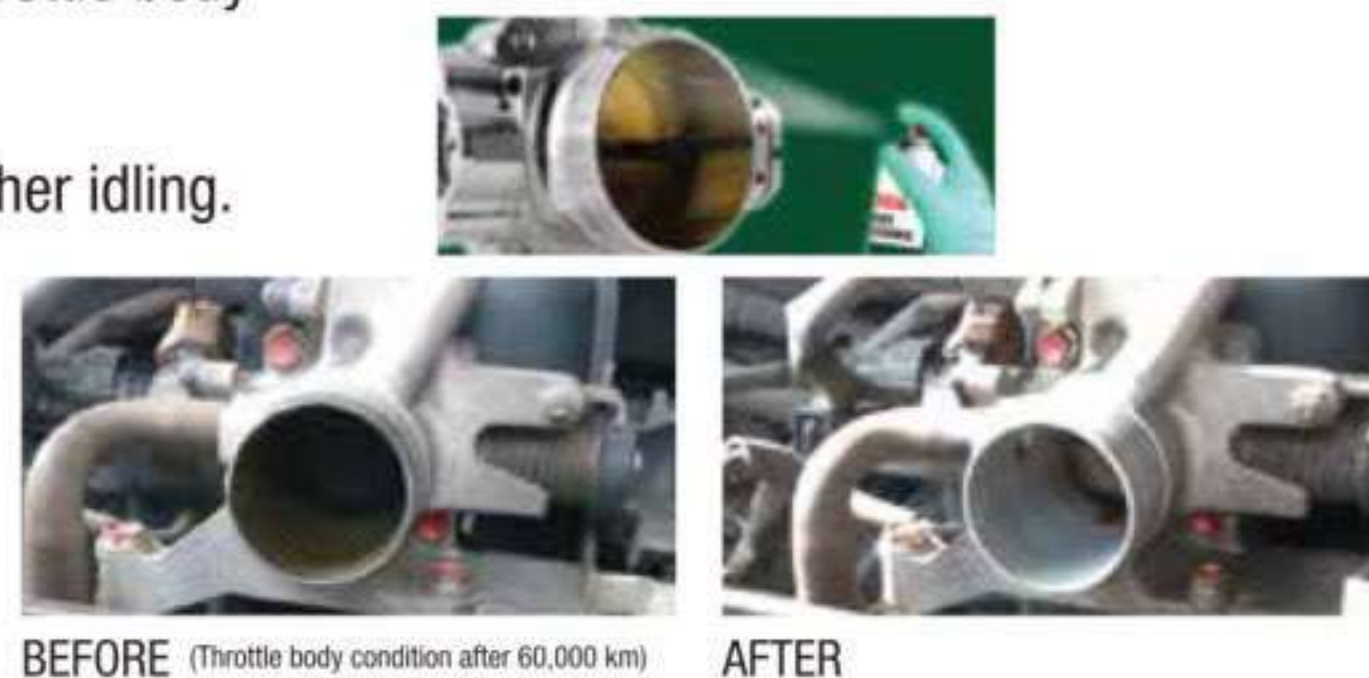
BEFORE (Throttle body condition after 60,000 km) AFTER
